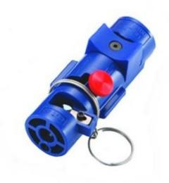
The Times Microwave Systems CST-400 Cable Preparation Tools is designed for EZI Fit crimp and clamp connectors. This combination tool reduces the need for braid trimming and provides excellent dielectric removal for easy connector termination. With this tool you can accurately strip and prepare LMR400 cable for precise connector attachment when using non-solder type Ezi-Fit Clamp or Crimp connectors. This model includes a built-in deburring tool eliminating the need for a separate tool.
