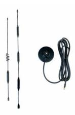
Portable magnetic base antenna provides high gain and versatility for GSM, 3G, 4G and 5G services. Constructed with a two-piece steel radiator and detachable magnetic base. Comes with a 5 meter LMR200 grade low loss cable terminated with SMA Male connector.
