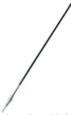
This rugged outdoor Omni Bull Bar antenna has a black fibreglass radiator and stainless steel spring. Designed for use on vehicles, the wide band frequency range of 690 to 2700MHz provides versatility for connections to 3G, 4G, 5G NR services across Australia. Comes with a 5 meter LMR195 grade cable.
