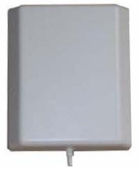
These directional panel antennas are designed for permanent installation indoor or outdoor. They are wideband supporting 690-4000MHz frequencies for 3G, 4G and 5G cellular networks. Applications include repeater coverage antenna, pole-mounted base station antenna and desktop induction pad. Wideband capability provides compatibility across all Australian mobile phone networks.
