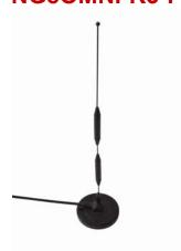
Portable and compact magnetic base antenna provides high gain and versatility for 3G, 4G, 5G NR services. Constructed with steel radiator and plastic detachable base, which contains a magnet and protective rubber boot. Comes with a 5 meter LMR195 grade cable terminated with FME Female connector.
