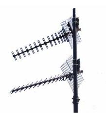
Comprises a pair of antennas. These high performance twin element Dual Yagi/Grid MiMo directional antennas provide a high signal gain for 3G, 4G and 5G NR devices that have two antenna connectors. The pair of antennas come with SMA Male pigtail cable and 45° polarisation mounting brackets.
