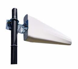
This antenna offers exceptional performance and versatility with 70 degree wide beam and wide band (690-5000MHz) for GSM/3G/4G/5G services. Log Periodic Directional Antenna (LPDA) design is compact and maintains virtually linear high gain across the specified frequency bands. Comes with a 6 meter LMR200 grade cable terminated with SMA Male connector.
