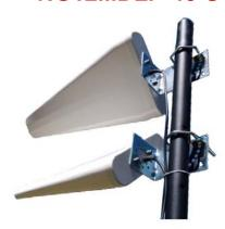
This Wide Band MiMo Antenna comprises dual Log Periodic Directional Antenna (LPDA) and offers exceptional performance and versatility with 70 degree wide beam and wide band (698-5000MHz) for GSM/3G/4G/5G services. LPDA design is compact and maintains virtually linear high gain across the specified frequency bands. The pair of antennas come with 45° polarisation mounting brackets and two 6 meter LMR200 grade cables terminated with SMA Male connectors.
